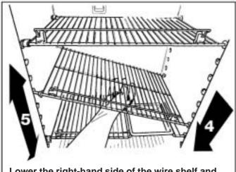
Lower the right-hand side of the wire shelf and let the left-hand side slide out of the holes in the wall.
